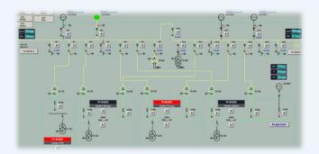
Two levels of load shedding are used. The first level, by detection of an under frequency consists of step by step shedding of HV breakers, according to the preset priority, which continues until the frequency returns to normal.
